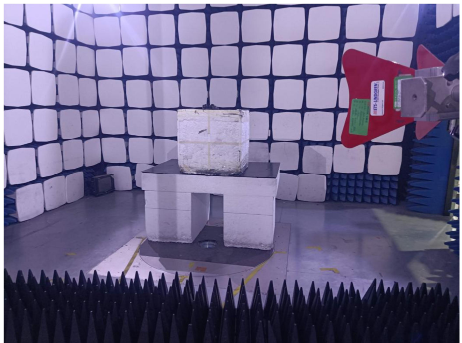
Radiation Emission Test Setup (1GHz to 18GHz)
