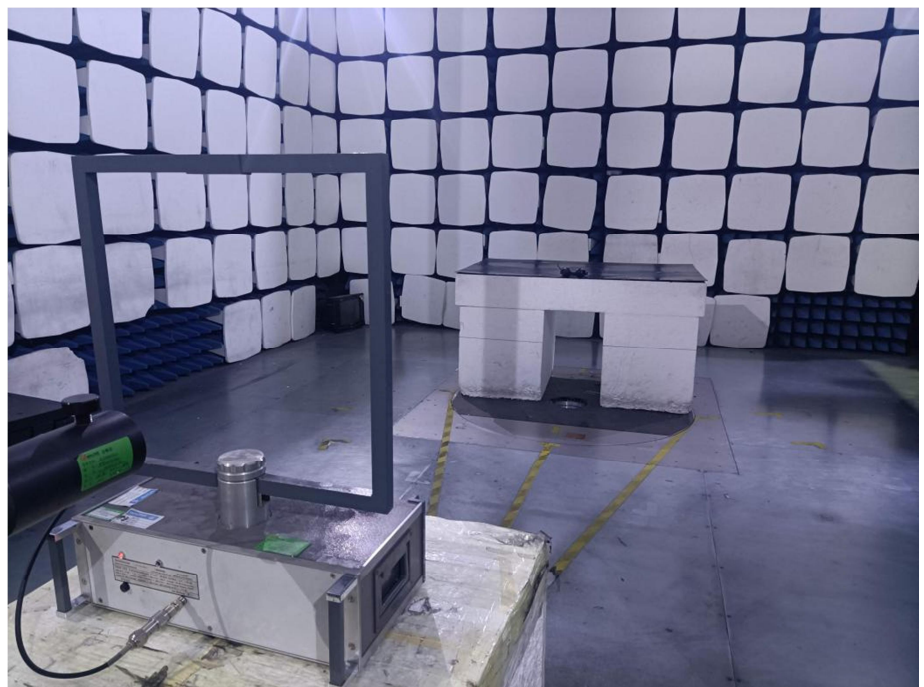
Radiation Emission Test Setup (Below 30MHz)
