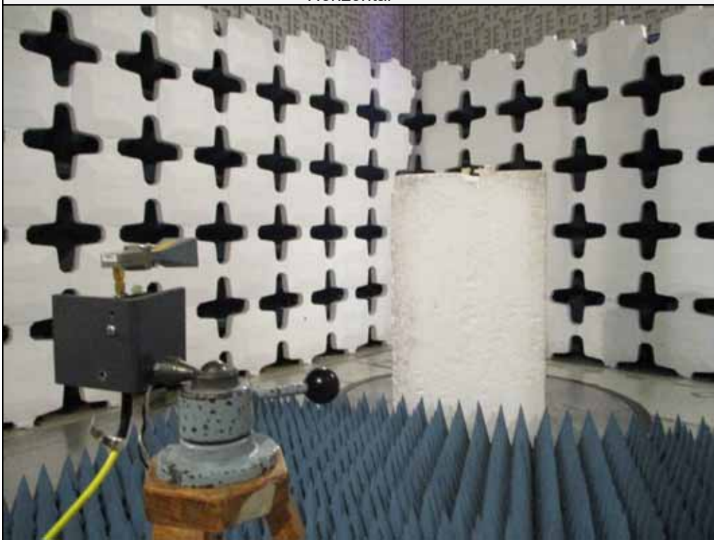
Test Setup for Spurious Radiated Emissions, 18-25GHz – Antenna Polarization Vertical
