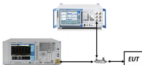
Figure 7-2. Test Instrument & Measurement Setup
