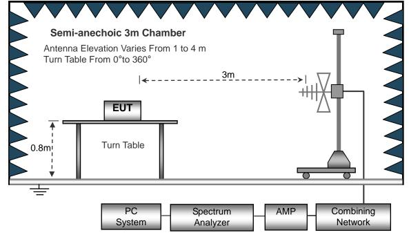
(C) Radiated Emission Test-Up Frequency Above 1GHz
