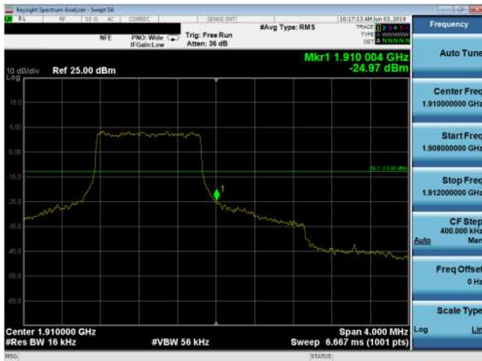
Plot 7-119. Upper Band Edge Plot (Band 2 - 1.4MHz QPSK - Full RB Configuration)
