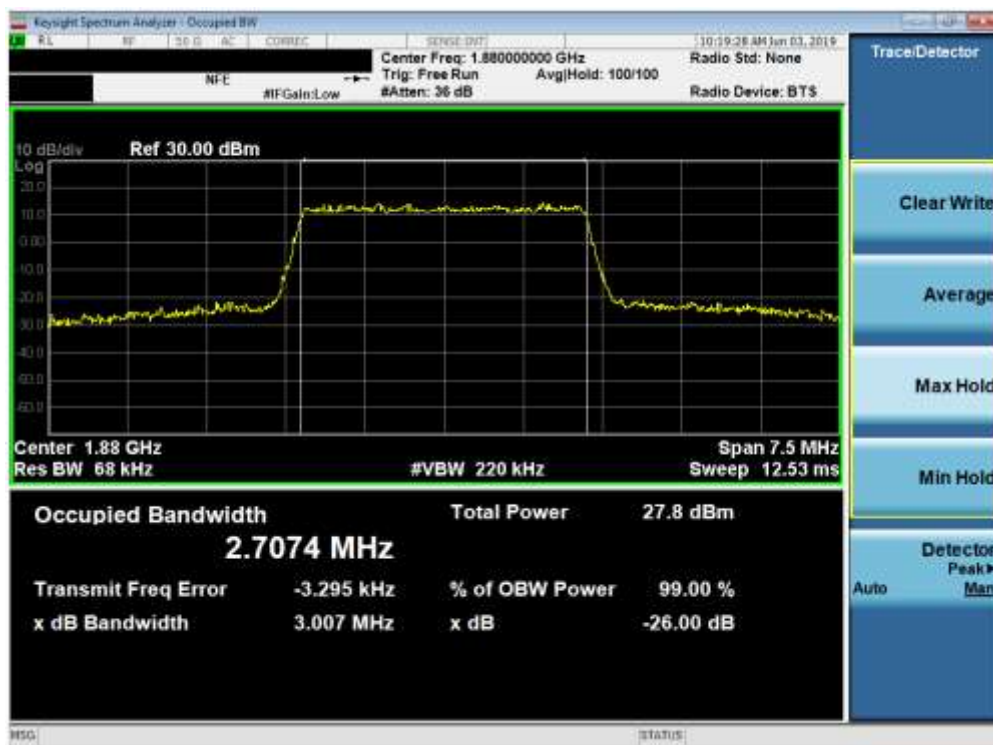
Plot 7-32. Occupied Bandwidth Plot (Band 2 - 3.0MHz 16-QAM - Full RB Configuration)
