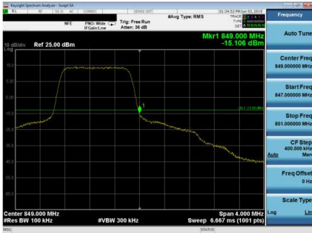
Plot 7-86. Upper Band Edge Plot (Band 5 - 1.4MHz QPSK - Full RB Configuration)
