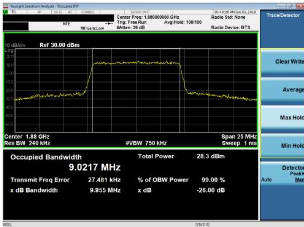
Plot 7-36. Occupied Bandwidth Plot (Band 2 - 10.0MHz 16-QAM - Full RB Configuration)
