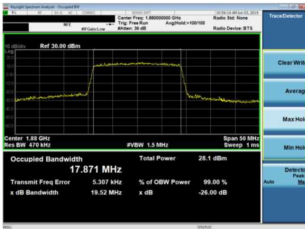
Plot 7-40. Occupied Bandwidth Plot (Band 2 - 20.0MHz 16-QAM - Full RB Configuration)
