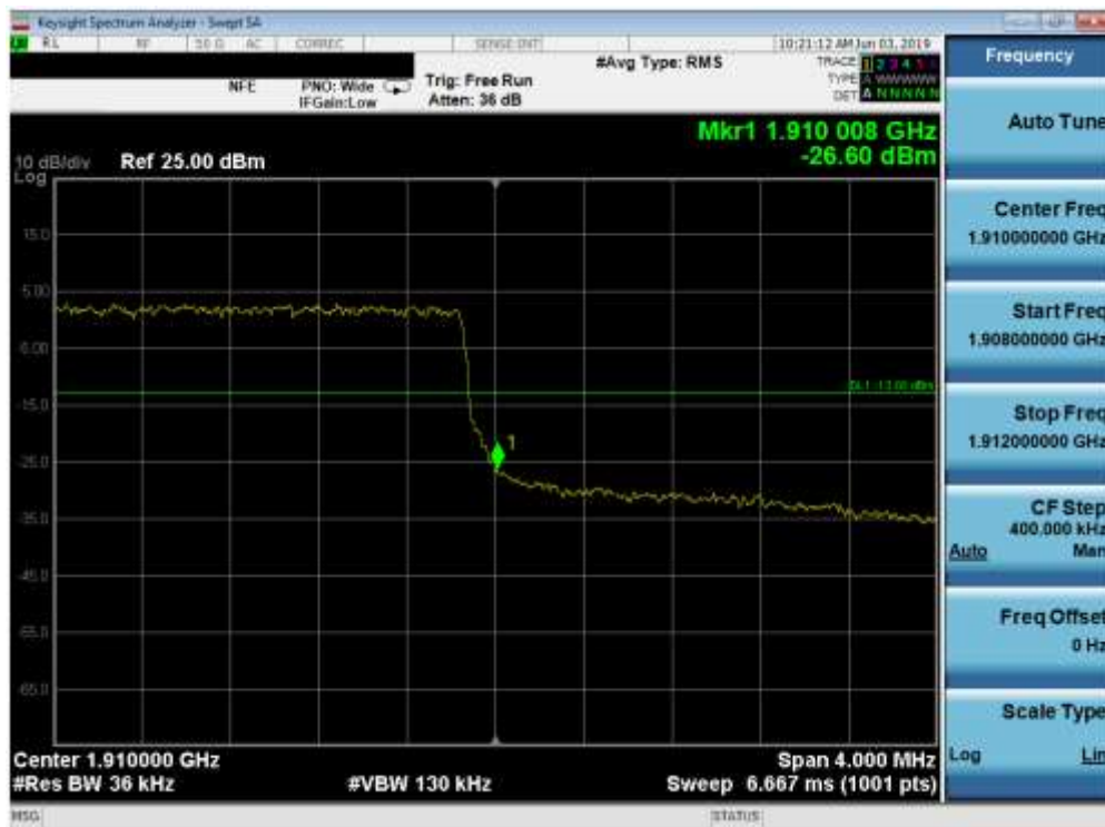
Plot 7-123. Upper Band Edge Plot (Band 2 - 3.0MHz QPSK - Full RB Configuration)
