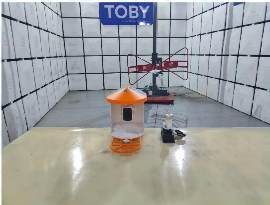
Photo of Setup for Radiated Emission (30MHz~1GHz)
