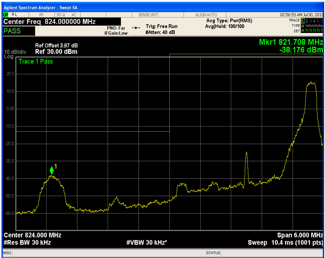
LTE Band41 QAM16 BW=5MHz Channel=41215 RB Size=25 Position=#0
