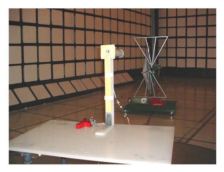
Radiated Emissions @ 3 m, Orthogonal Position 2 EUT with 15.0 dBi Yagi Antenna and 8.6 dB Assembly Cable Loss
