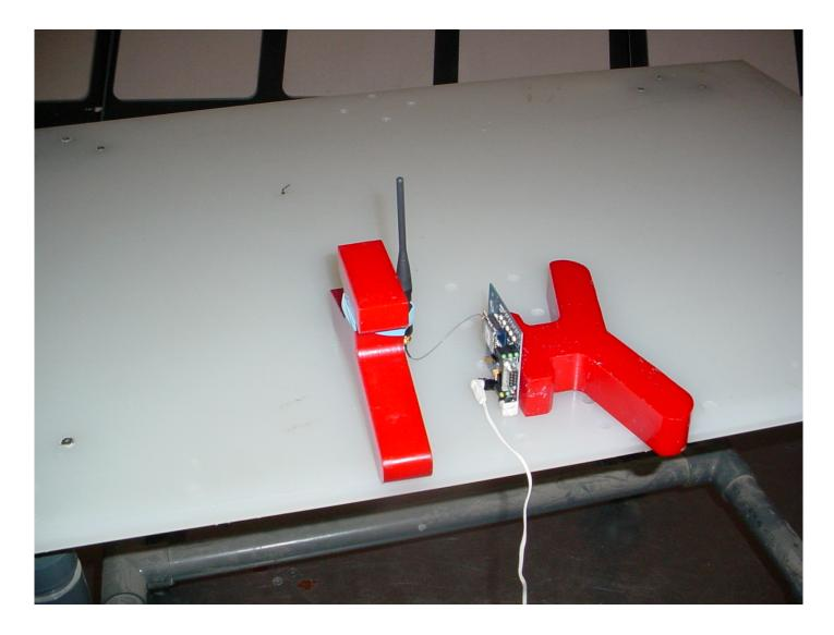
Radiated Emissions @ 3 m EUT with 2.1 dBi Dipole Antenna and 0.53 dB Assembly Cable Loss
