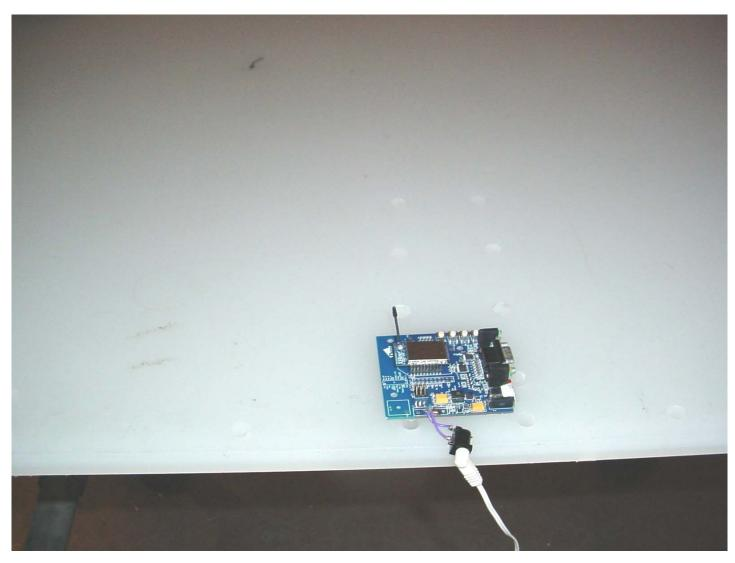
Radiated Emissions @ 3 m EUT with 1.5 dBi Monopole (Integrated Whip) Antenna
