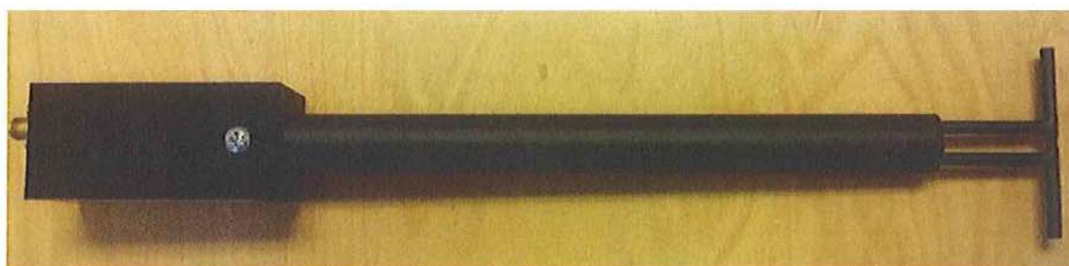
Figure 1 – MVG COMOSAR Validation Dipole
