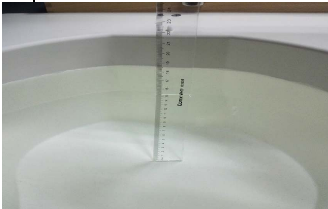
The Body Liquid of 2400MHz (15.4cm)
