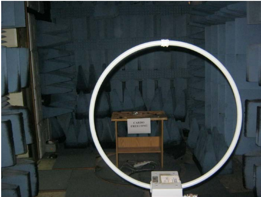
Figure 6. Radiated Emission Test – 9kHz-30MHz
