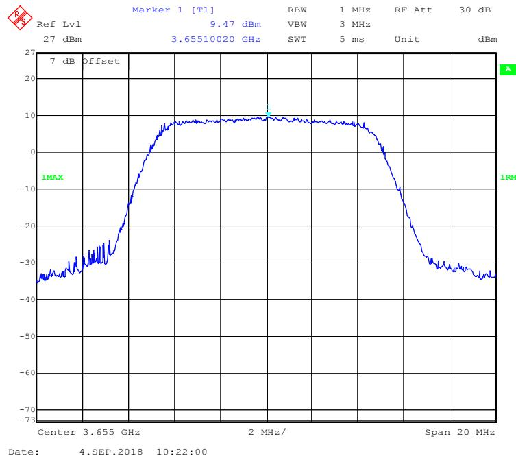
**16-QAM (10 MHz) - Peak Power Density, Middle channel**
