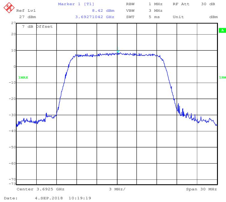
**QPSK (15 MHz) - Peak Power Density, Low channel**
