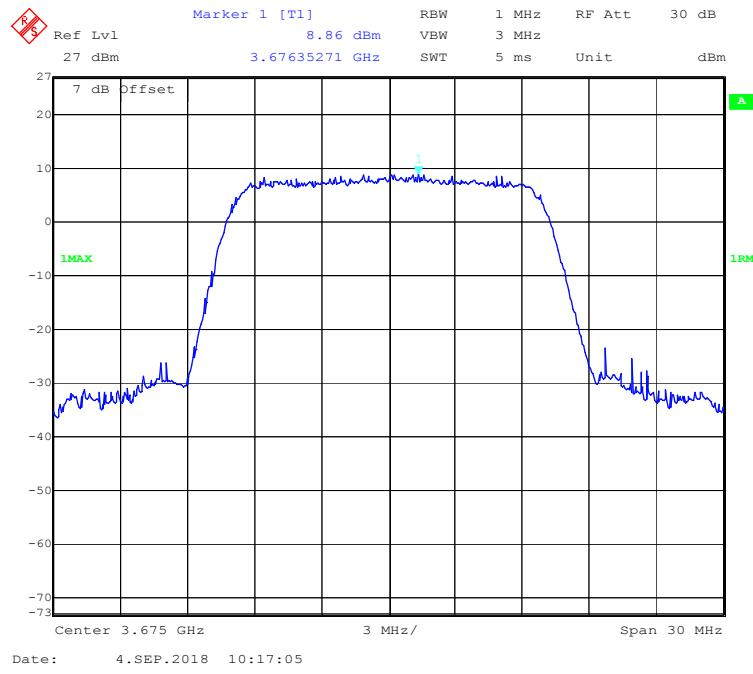
**QPSK (15 MHz) - Peak Power Density, High channel**
