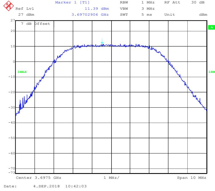
**QPSK (10 MHz) - Peak Power Density, Low channel**
