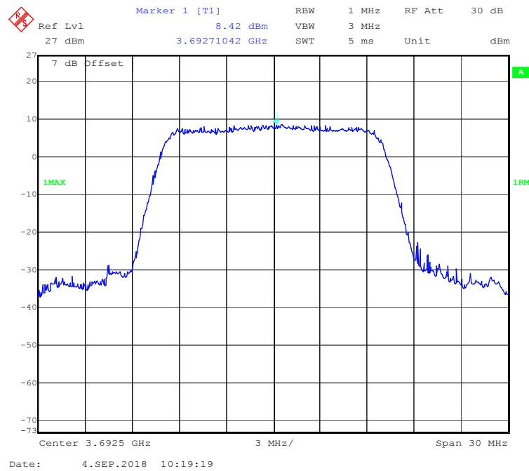
**QPSK (20 MHz) - Peak Power Density, Low channel**
