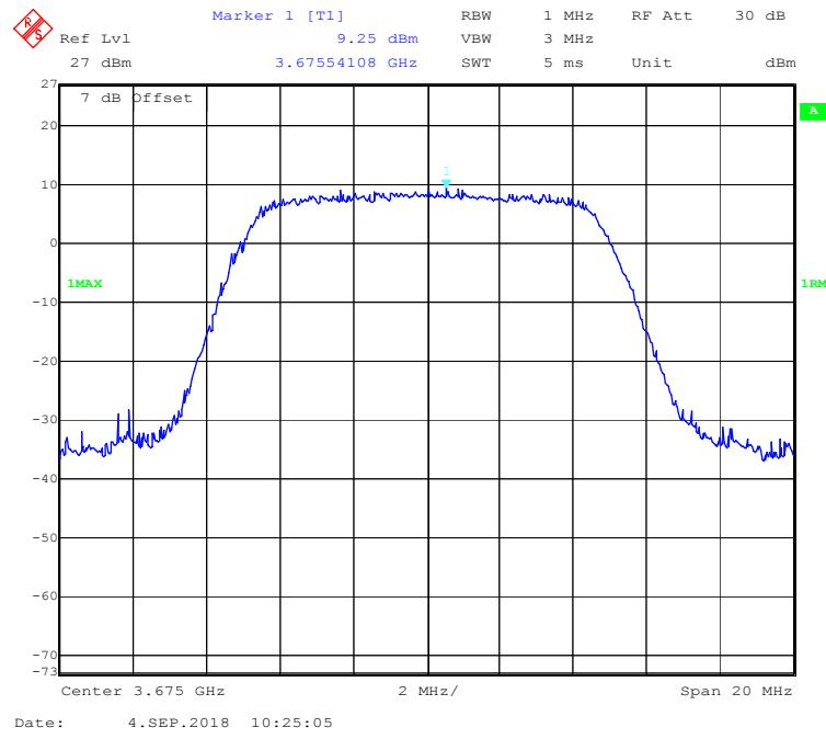
**QPSK (10 MHz) - Peak Power Density, High channel**
