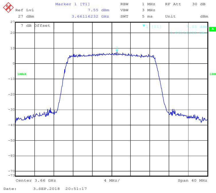
**16-QAM (20 MHz) - Peak Power Density, Middle channel**
