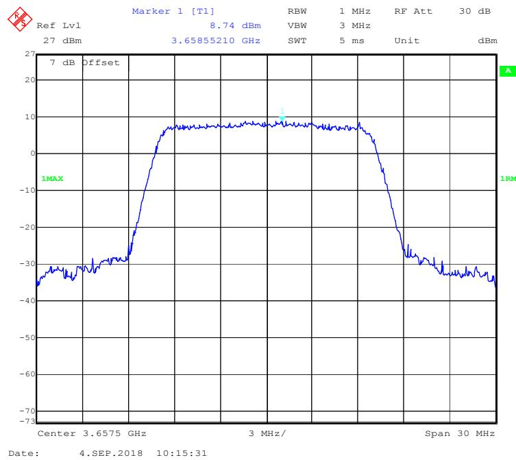
**16-QAM (15 MHz) - Peak Power Density, Middle channel**
