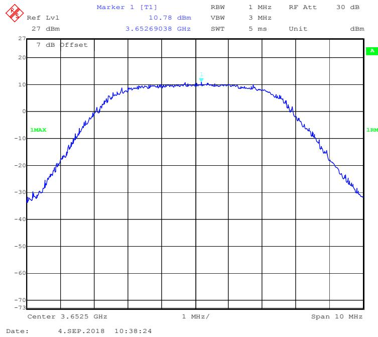
**16-QAM (5 MHz) - Peak Power Density, Middle channel**
