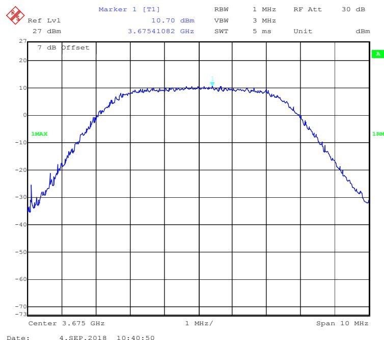
**QPSK (5 MHz) - Peak Power Density, High channel**
