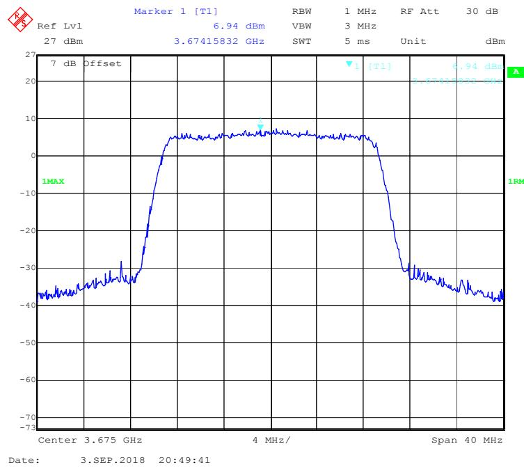
**QPSK (20 MHz) - Peak Power Density, High channel**
