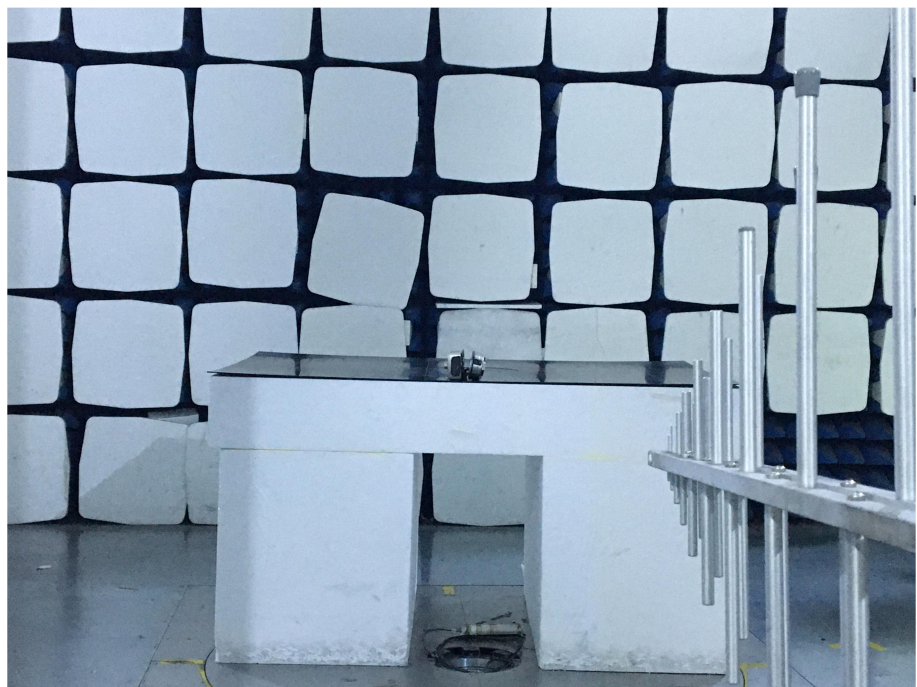
Radiation Emission Test Setup (30MHz to 1GHz)
