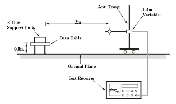
The radiated emission tests were performed in the 3 meters chamber B test site, using the setup accordance with the FCC MP - 5. The specification used was the FCC part 18.
