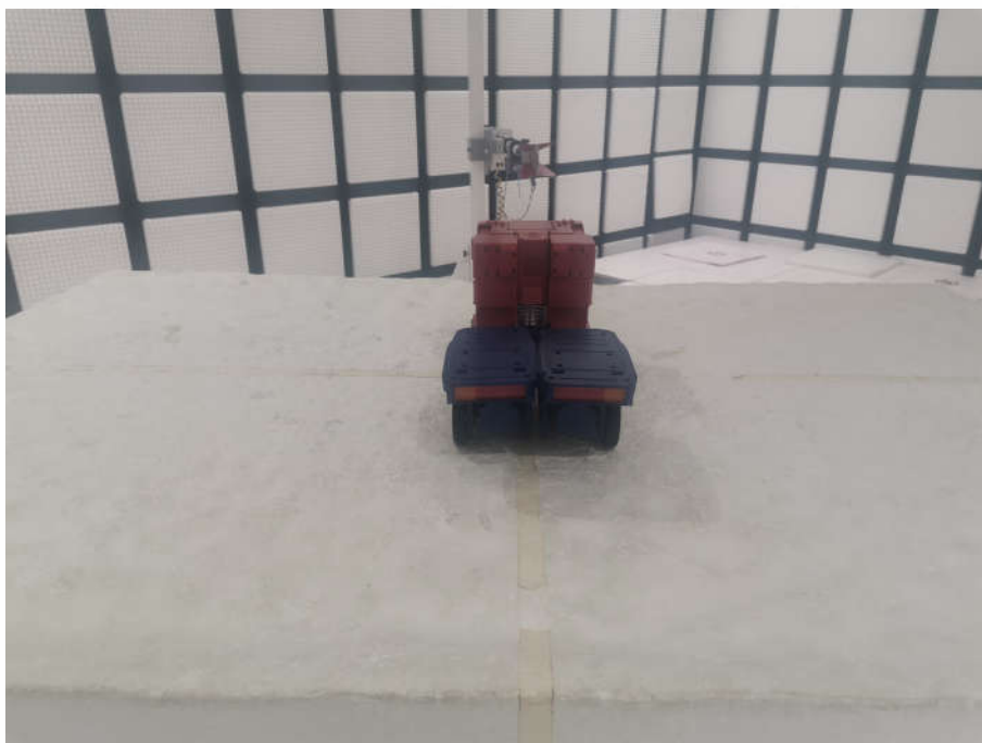
Radiated spurious emission Test Setup-2(Above 1GHz)
