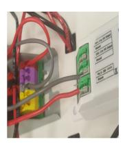
Step 3, Connect purple dimming wires
