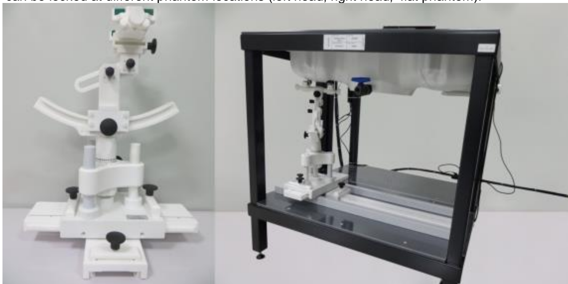
Device holder supplied by SATIMO
