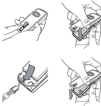
Put the strap through the hook inside and at the bottom of the phone. Pull the strap to lock it into place.
