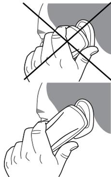
The antenna is integrated in your phone, under the back cover at the top. Avoid putting your fingers on this area when the phone is switched ON. If your fingers obstruct the antenna, the phone may have to operate with a higher power level than usual; decreasing its efficiency quickly. It could also affect the quality of your communications.
