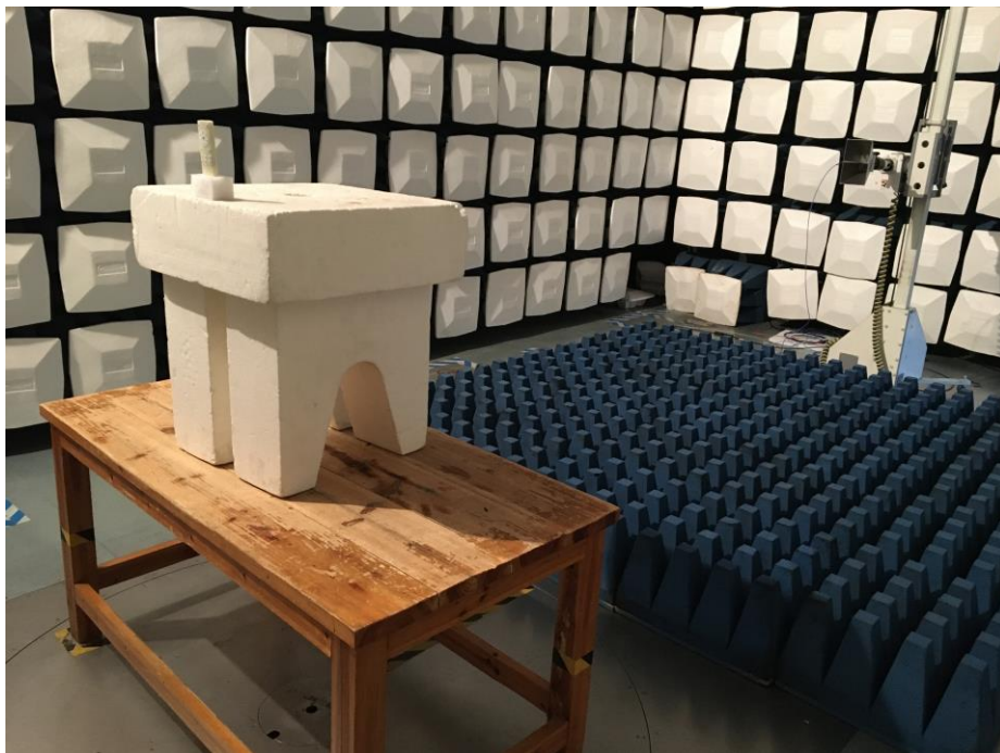
Test Setup For Radiated Emission (Above 1GHz)
