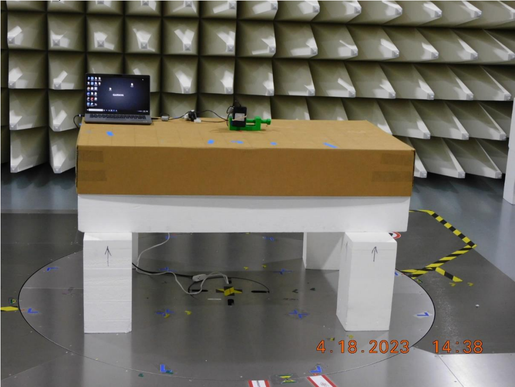
Figure RE14.2: EUT test setup, front view (Antenna X Orientation)
