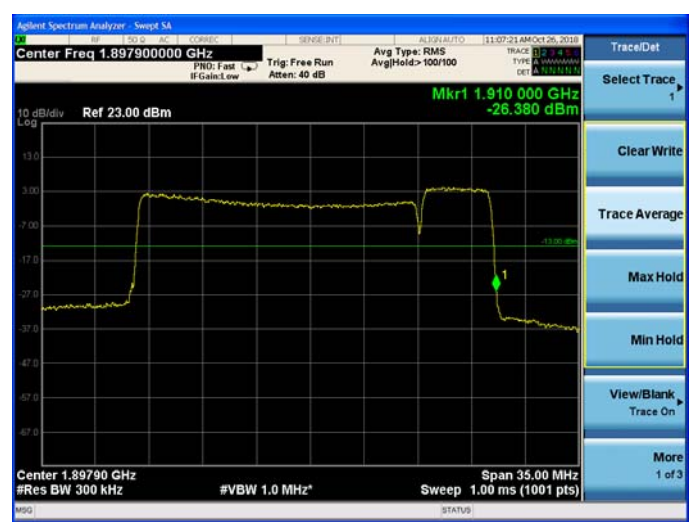
CA_2C 20MHz+20MHz QPSK RB=1#0+1#99 CH- High
