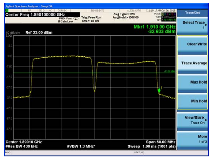
CA_2C 20MHz+5MHz 16QAM RB=1#0+1#24 CH- High
