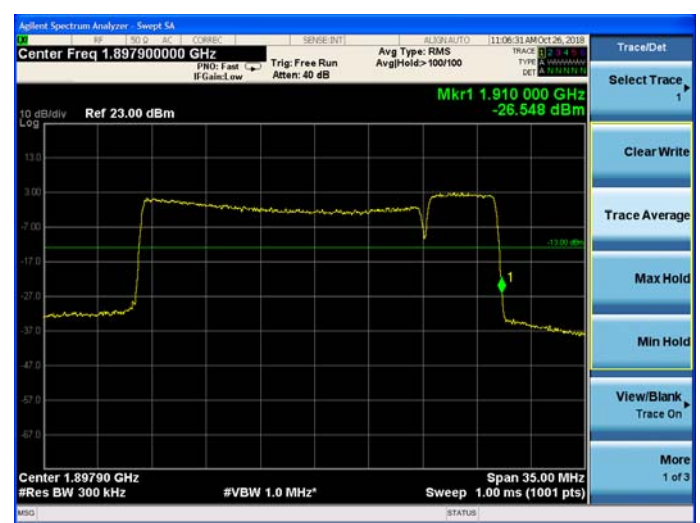
CA_2C 20MHz+5MHz 16QAM RB=100#0+25#0 CH-High
