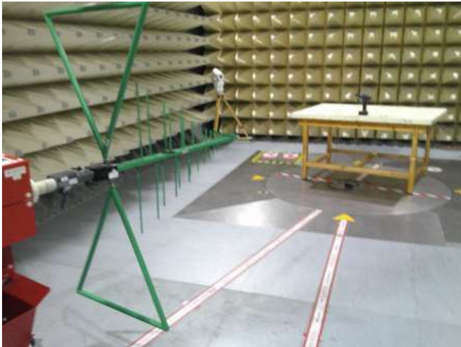
Photograph 1: Set-up for measurement of radiated emission
