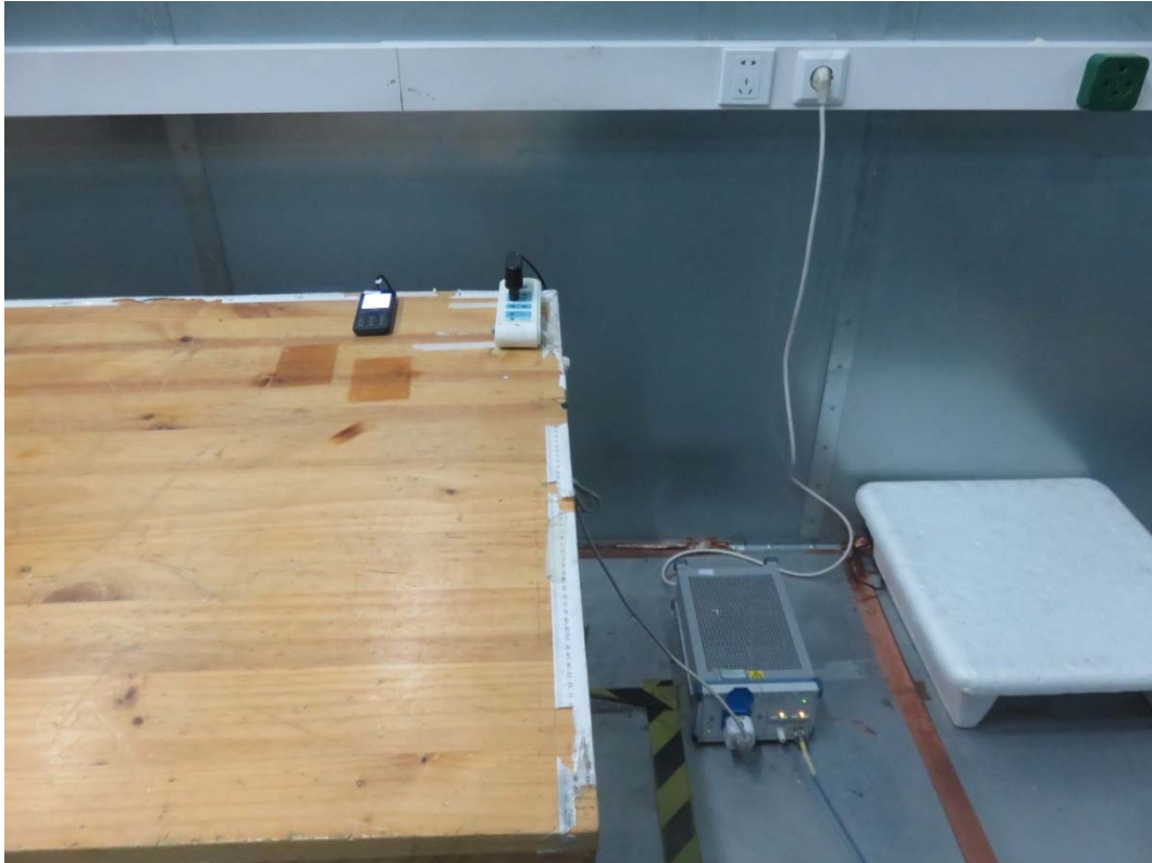
Picture 3 Conducted Emission Test Setup
