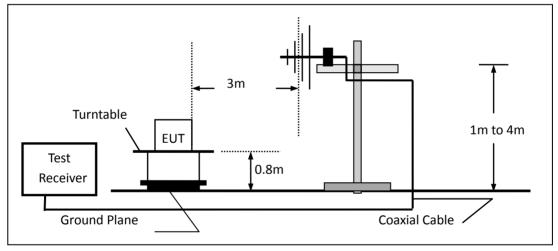
(c) For radiated emissions above 1000MHz
