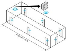
Example of placement of the Hub with 8 locks. AH40 can manage up to 64 locks
