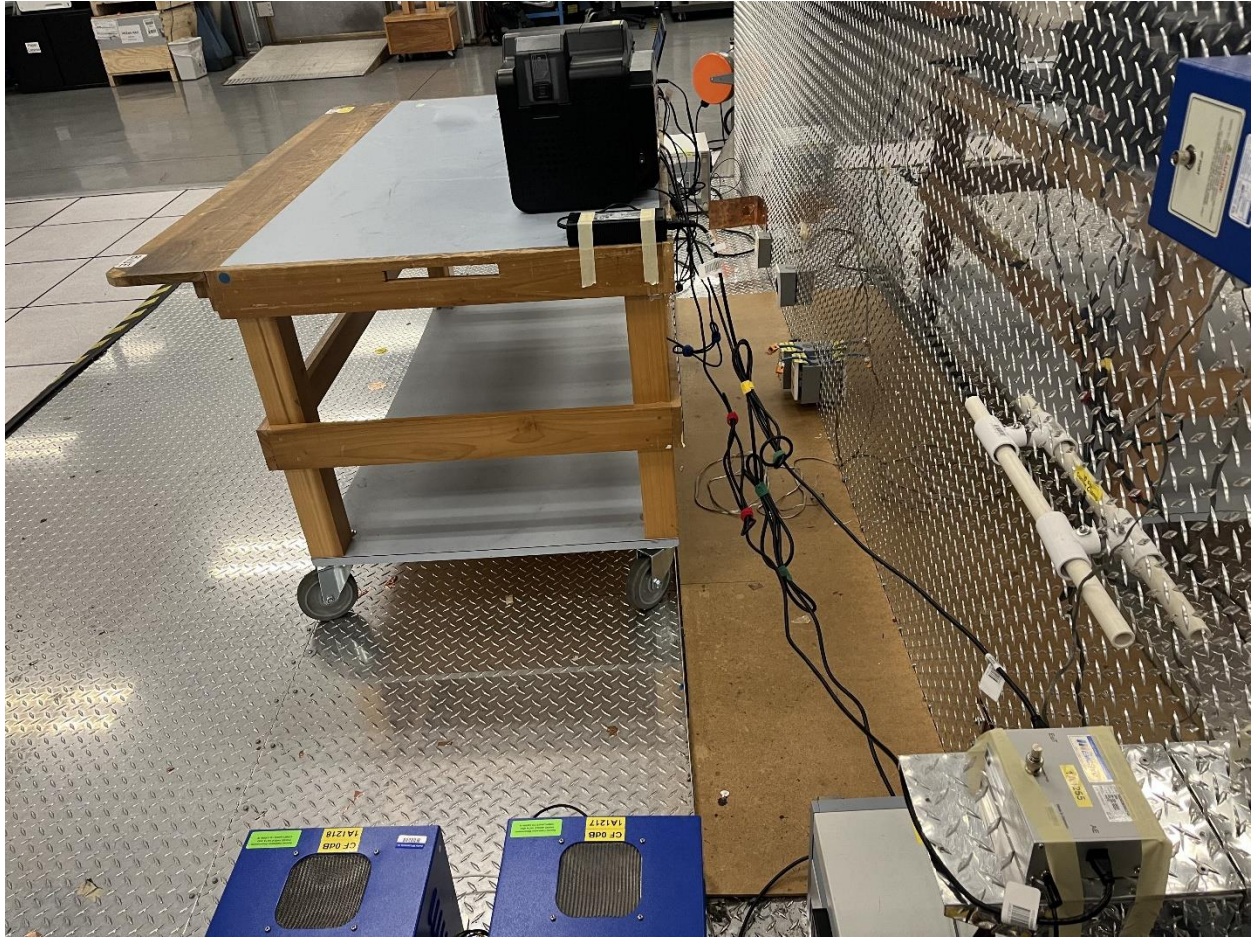
Conducted Emissions Side View
