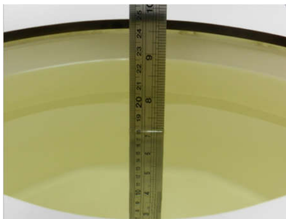
Fig 11.1 Photo of Liquid Height for Body SAR
