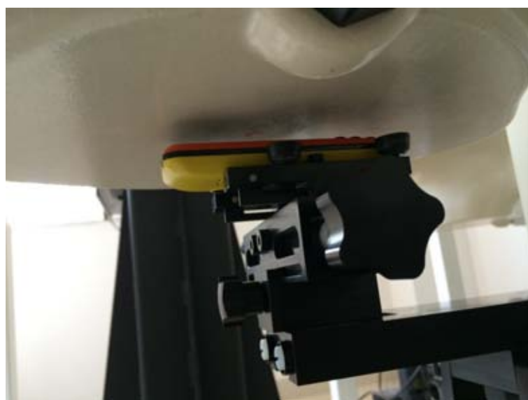
10mm Body-worn front Side Setup Photo
