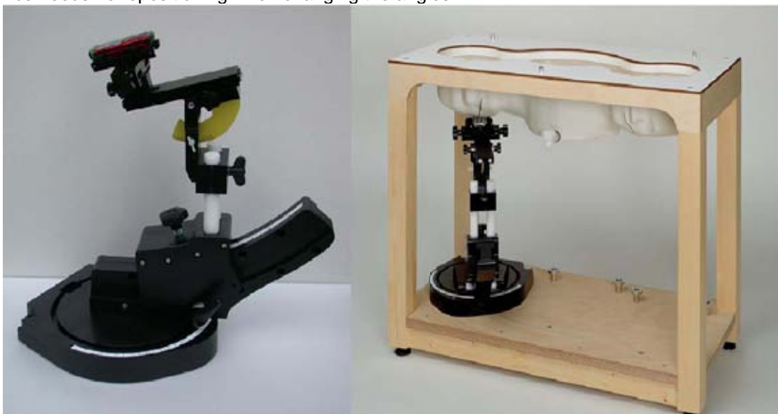
Device holder supplied by SPEAG
