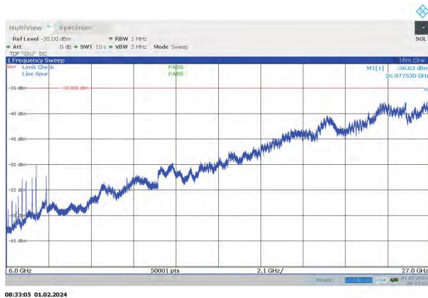
Spurious Emissions (6GHz – 27GHz ) - QPSK (2655 MHz) (Band 7 NB-IoT GB 10MHz Channel BW)
