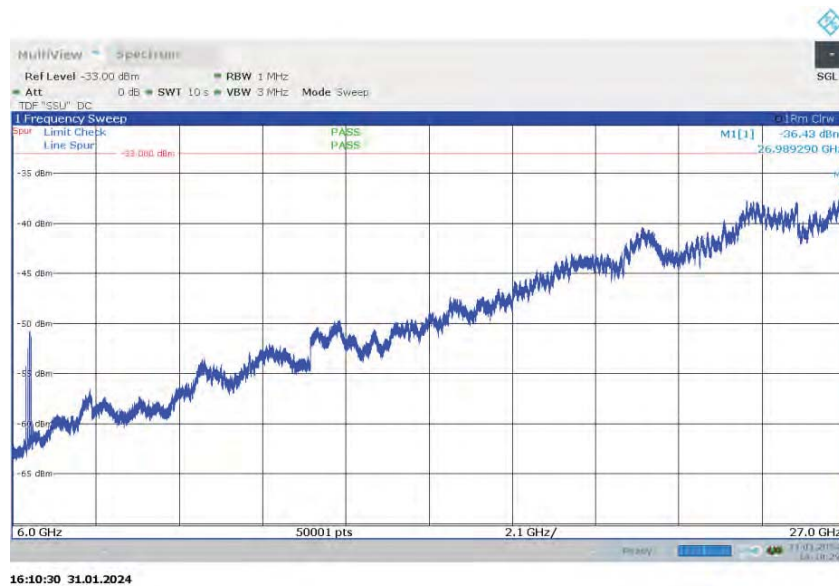
Spurious Emissions (6GHz – 27GHz) - QPSK (2110.2 MHz) (Band 66 NB-IoT SA 200kHz Channel BW)
