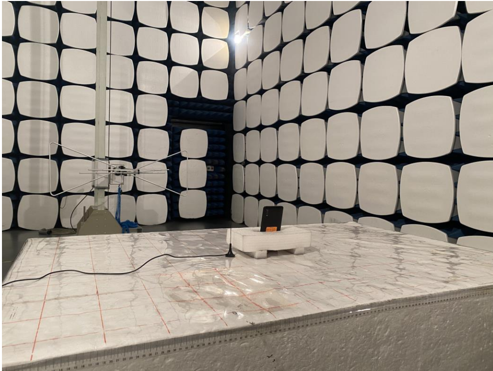
Radiated Spurious Emission Below 1GHz
