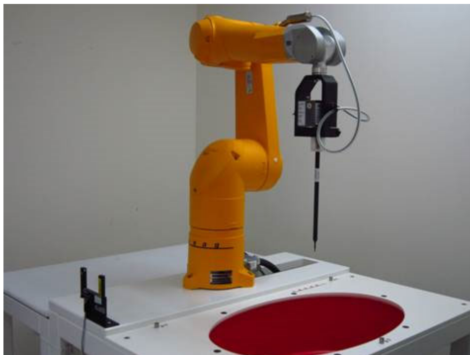
Fig.1 Photograph of the SAR measurement system
