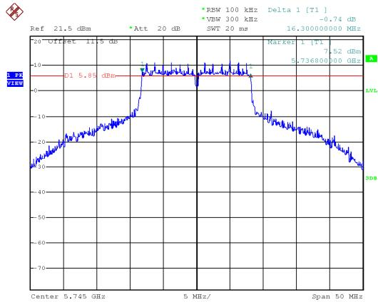
Modulation Standard: 802.11ac, VHT20 (6.5Mbps)
