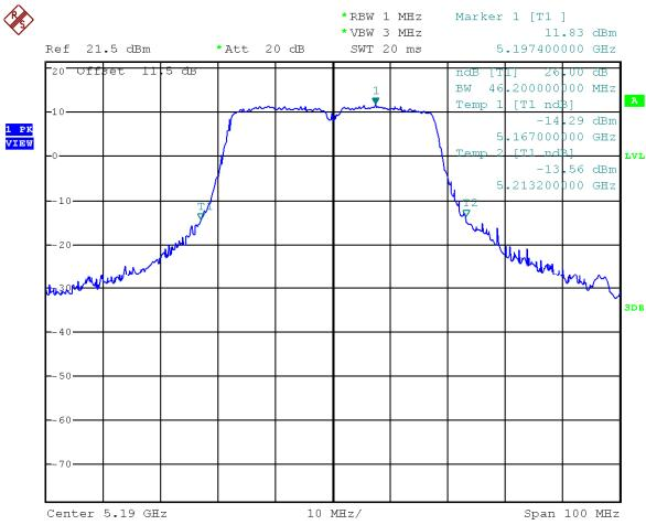
Modulation Standard: 802.11ac, VHT80 (29.3Mbps)
