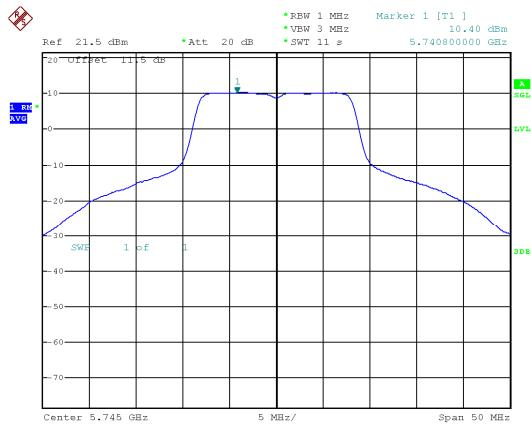
Modulation Standard: 802.11ac, VHT20 (6.5Mbps)
