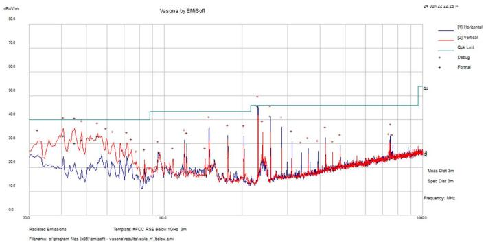
SA Correction Cord. **Antenna Turntable** Margin **Frequency Antenna** Limit Reading **Factor** Reading Height **Azimuth Comment** (dBuV/m) (dB)(MHz) **Polarity** (dBµV) (dB/m)  $(dB\mu V/m)$ (cm) (degrees) 230.52475 53.48 -7.65 45.84 Η 138 278 46 -0.16 QP 40.6785 39.48 -6.26 33.22 V 28 123 40 -6.78QP 45.11325 V 39.35 -9.18 30.17 101 352 40 -9.83 QP 257.65125 48.28 -6.73 41.56 Η 114 252 46 -4.44 QP 48.03 42.13 -10.63 31.51 V 135 70 40 -8.49 QP 55.19675 45 -11.98 33.01 V 100 97 40 -6.99 QP
