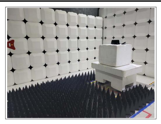
Test Setup Photo of Radiated Measurement (Above 1GHz)
