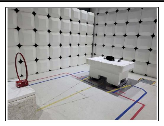
Test Setup Photo of Radiated Measurement (0.009 ~ 30MHz)
