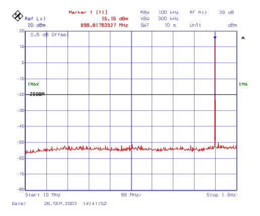
Plot # 20 : Spurious Emission Conducted at Antenna terminal, Low power setting Frequency: 898.5 MHz, Modulation: 2-Level 8kbps GMSK
