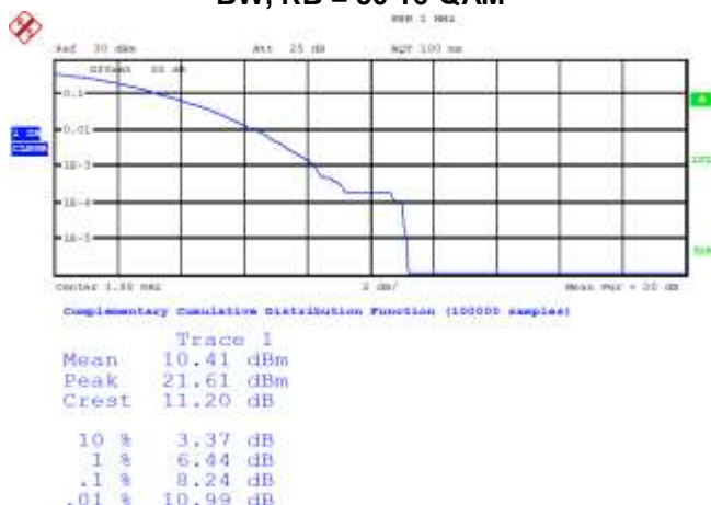
Figure 3-40a: Band 2, Mid Channel PAR, 10 MHz BW, RB = 50 16-QAM
