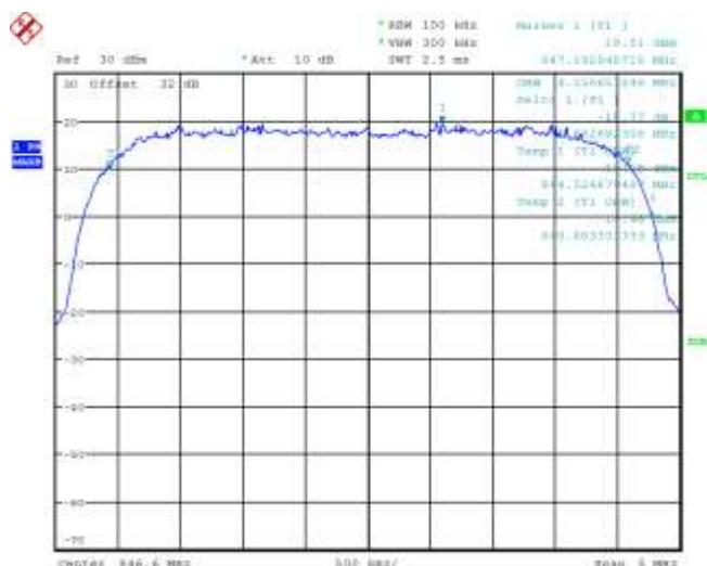
Figure 2-15a: Occupied Bandwidth, Band V High Channel
