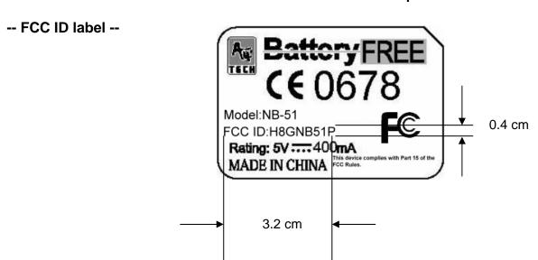
The remained portion of label statement required by FCC is attached in the user's manual.
