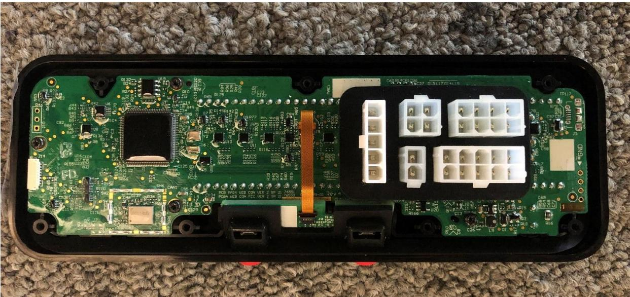
WC2 Controller Probe PCB Board - Front
