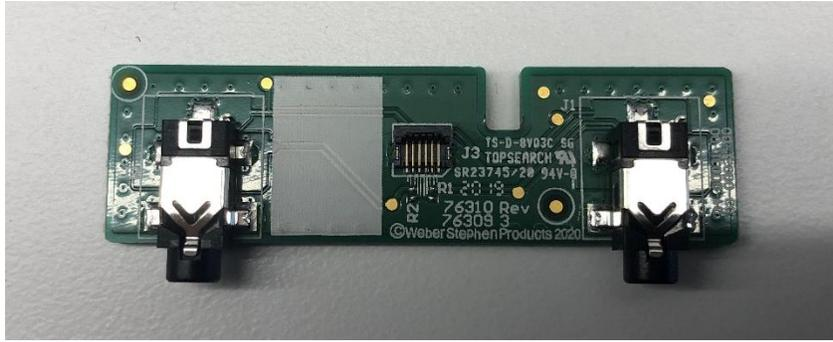
WC2 Controller Probe PCB Board - Back
