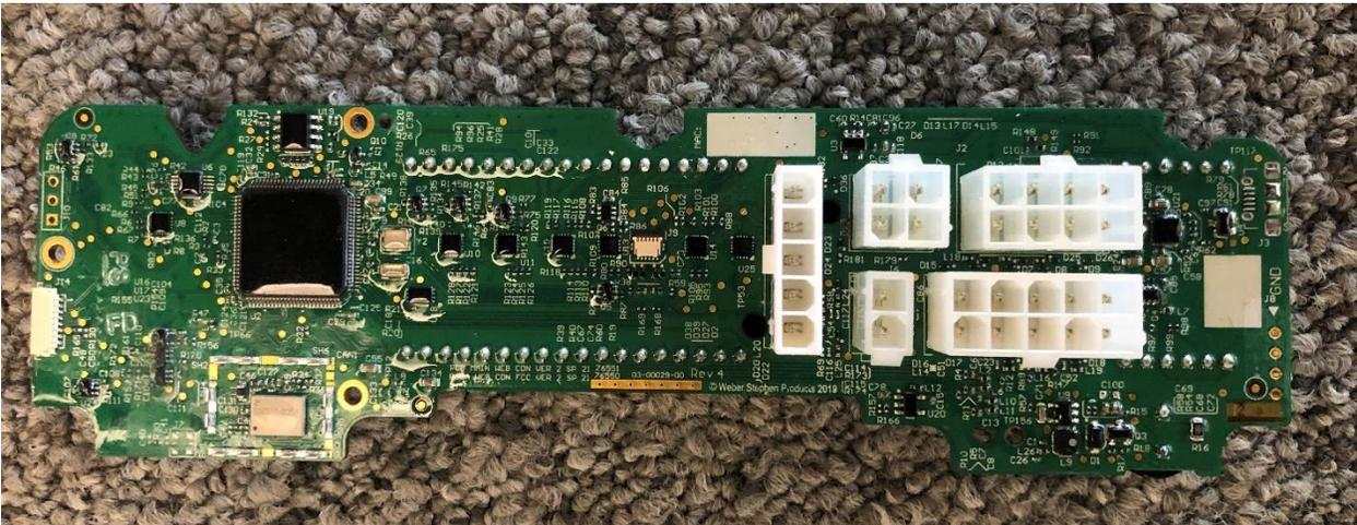
WC2 Controller PCB installed with Probe PCB Boards
