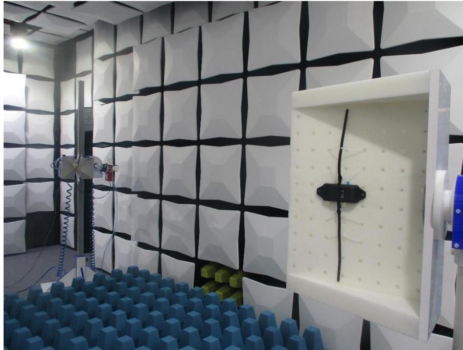
Test Setup: Radiated Measurements (1 GHz to 10 GHz)
