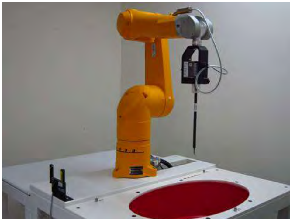
Fig.1 Photograph of the SAR measurement system
