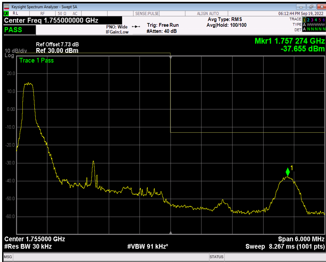
Band4 QPSK BW=3MHz Channel=20385 RB Size=1 Position=#Max
