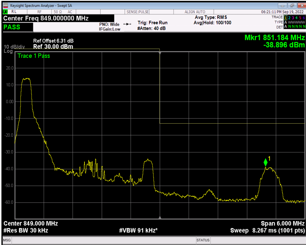
Band5 QPSK BW=3MHz Channel=20635 RB Size=1 Position=#Max
