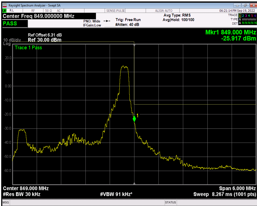
Band5 QPSK BW=3MHz Channel=20635 RB Size=15 Position=#0
