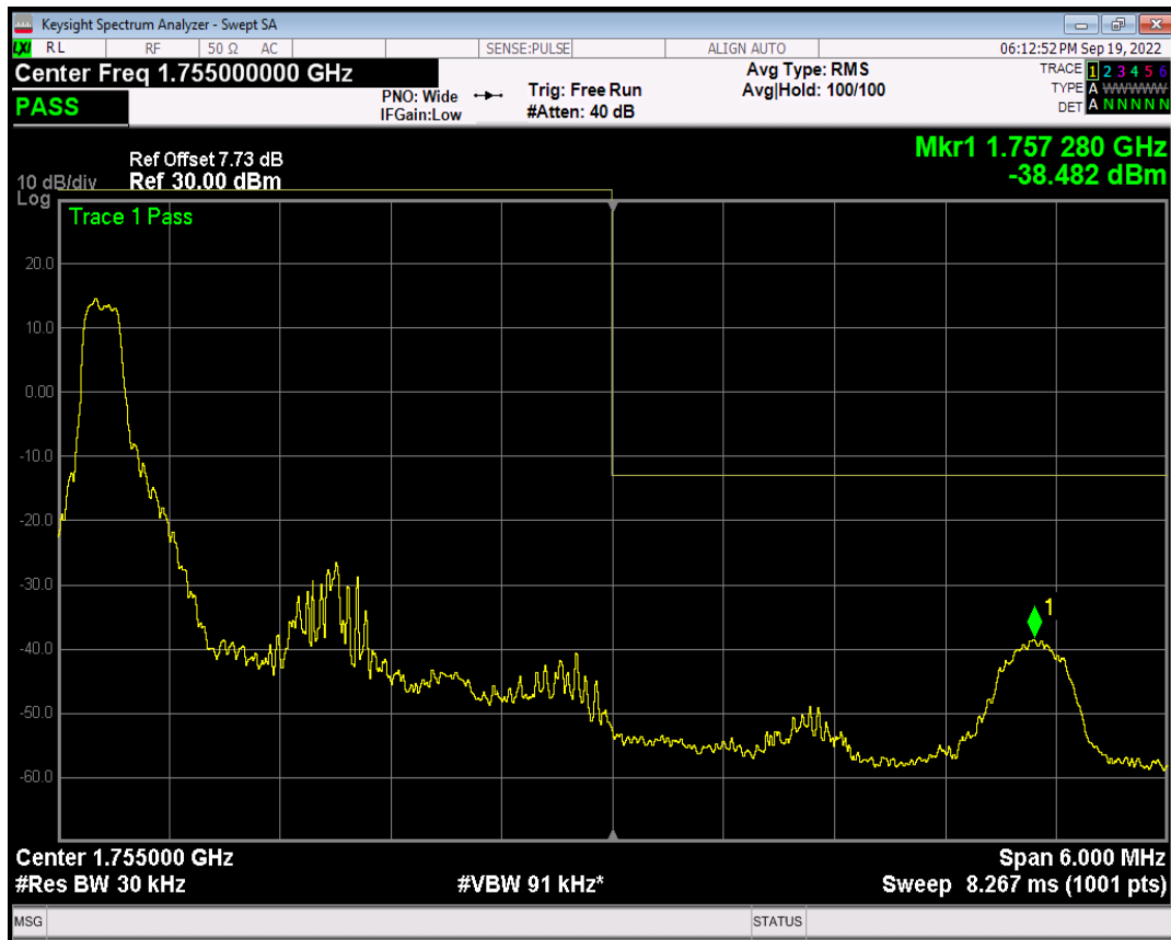
Band4 QAM16 BW=3MHz Channel=20385 RB Size=1 Position=#Max
