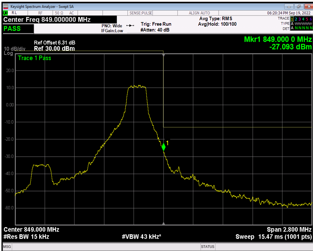
Band5 QPSK BW=1.4MHz Channel=20643 RB Size=6 Position=#0
