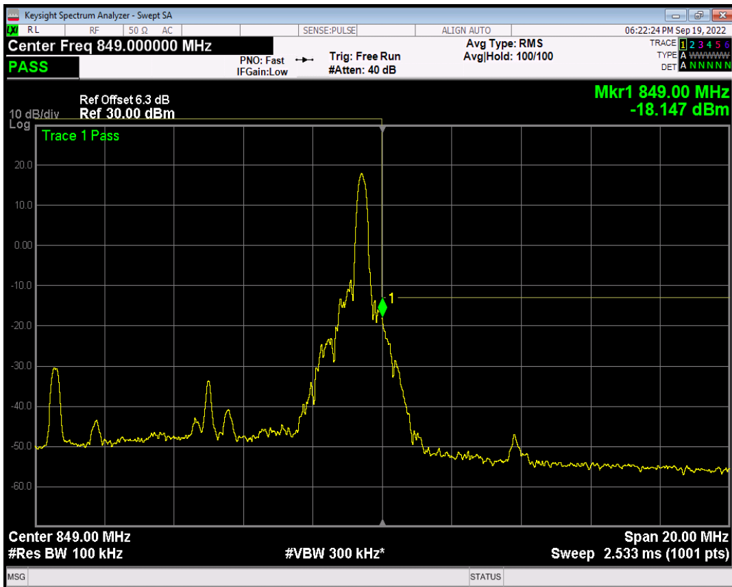
Band5 QAM16 BW=10MHz Channel=20600 RB Size=50 Position=#0
