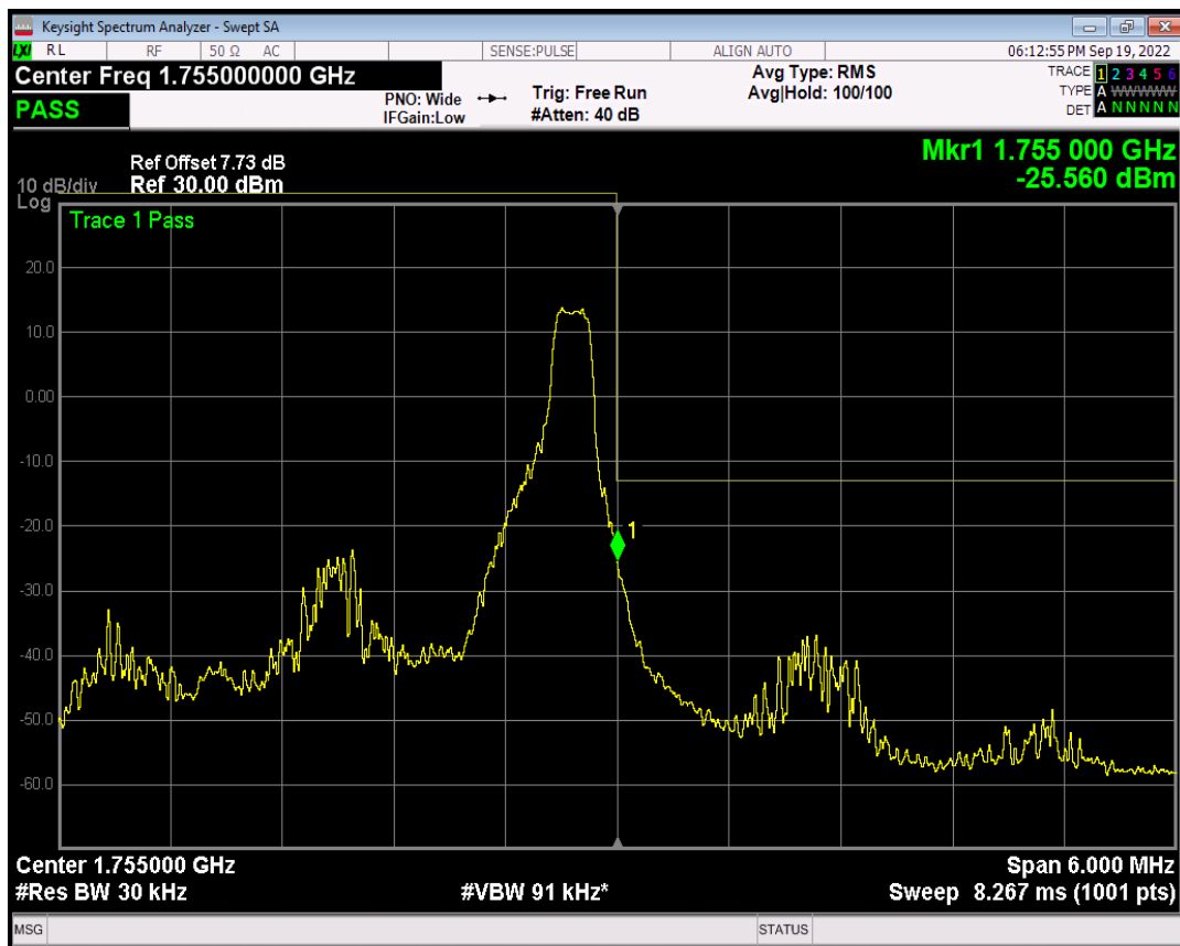
Band4 QAM16 BW=3MHz Channel=20385 RB Size=15 Position=#0
