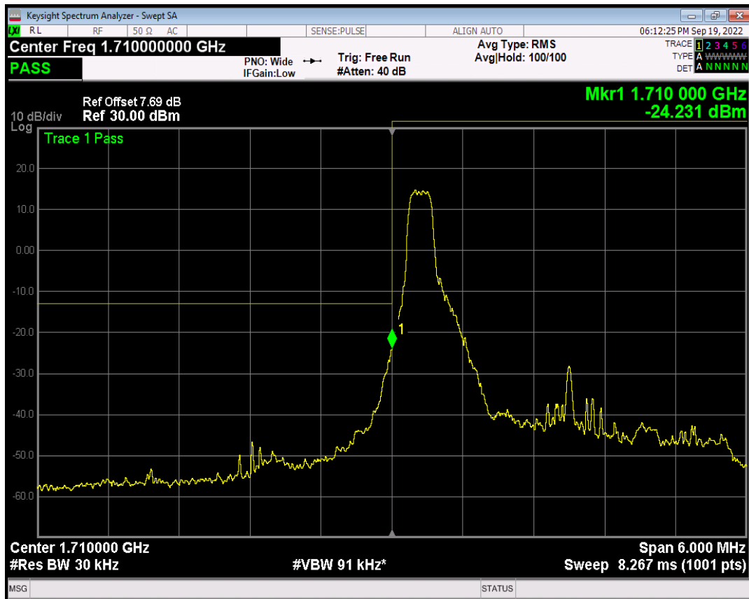
Band4 QPSK BW=3MHz Channel=19965 RB Size=1 Position=#Max
