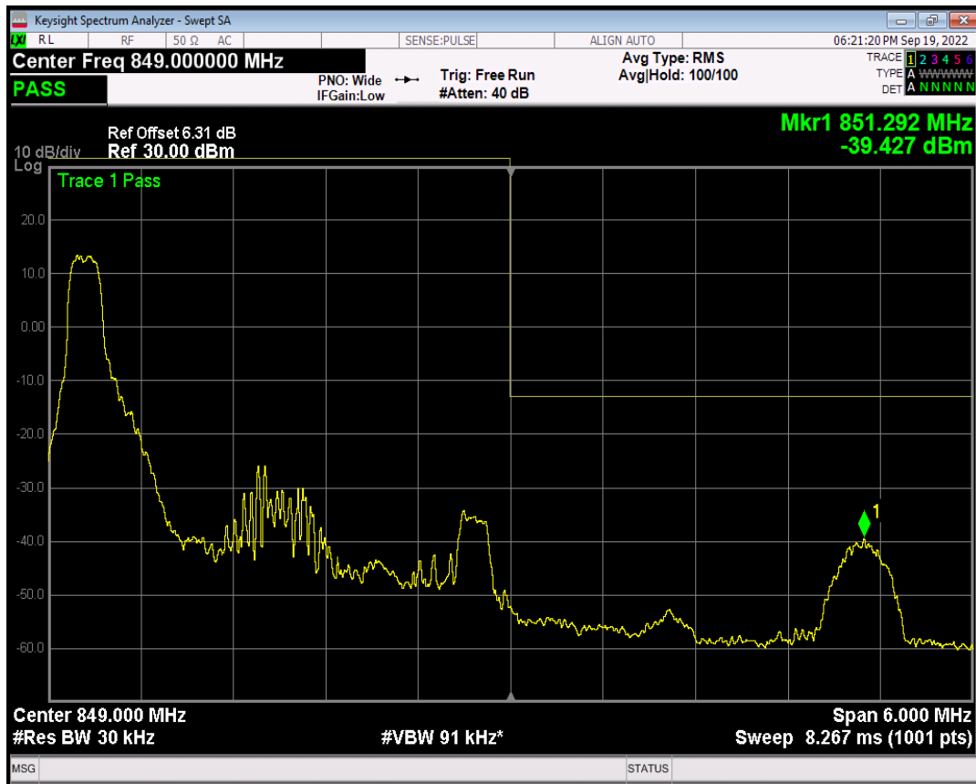
Band5 QAM16 BW=3MHz Channel=20635 RB Size=1 Position=#Max
