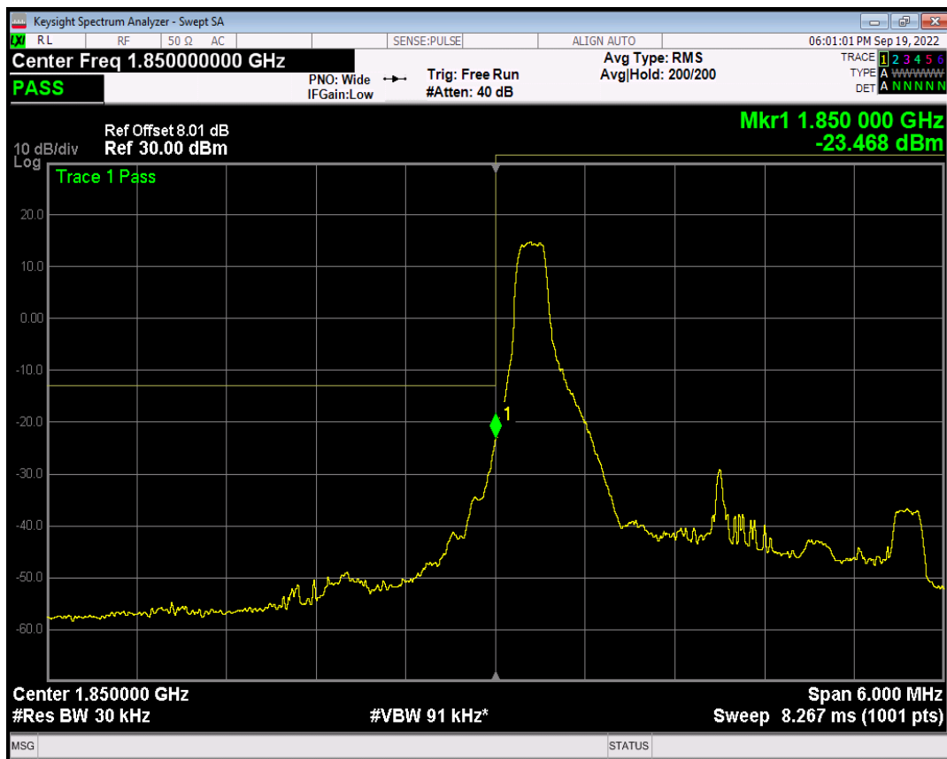
Band2 QPSK BW=3MHz Channel=18615 RB Size=1 Position=#Max
