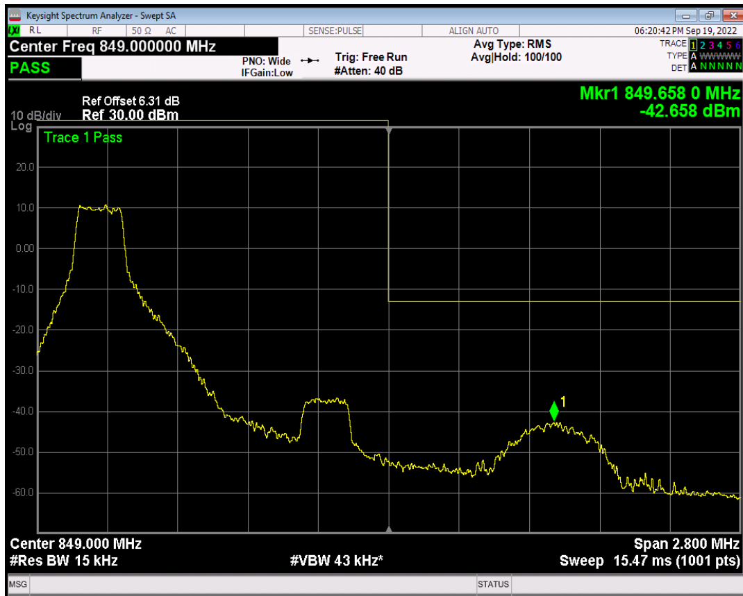
Band5 QAM16 BW=1.4MHz Channel=20643 RB Size=1 Position=#Max
