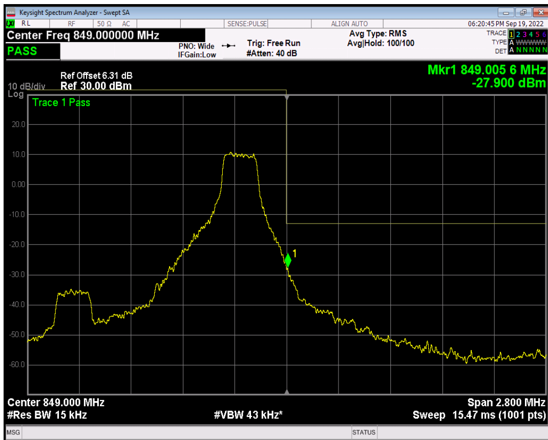
Band5 QAM16 BW=1.4MHz Channel=20643 RB Size=6 Position=#0
