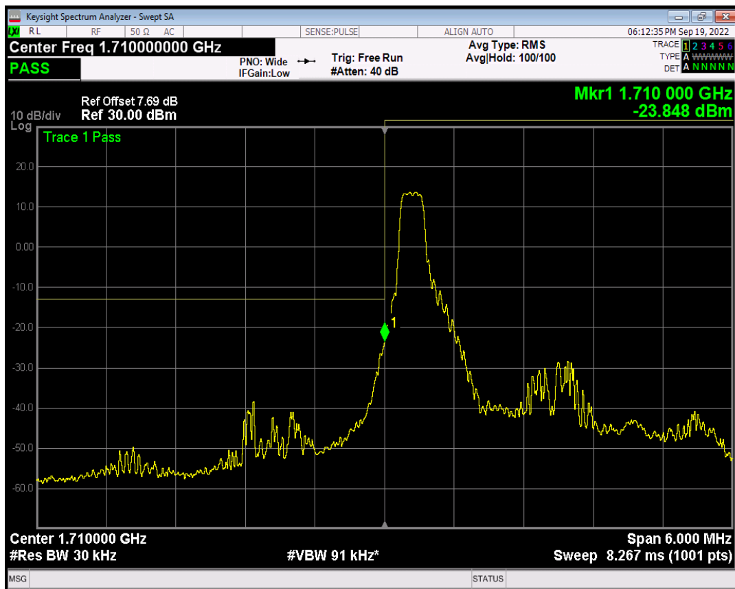
Band4 QAM16 BW=3MHz Channel=19965 RB Size=1 Position=#Max
