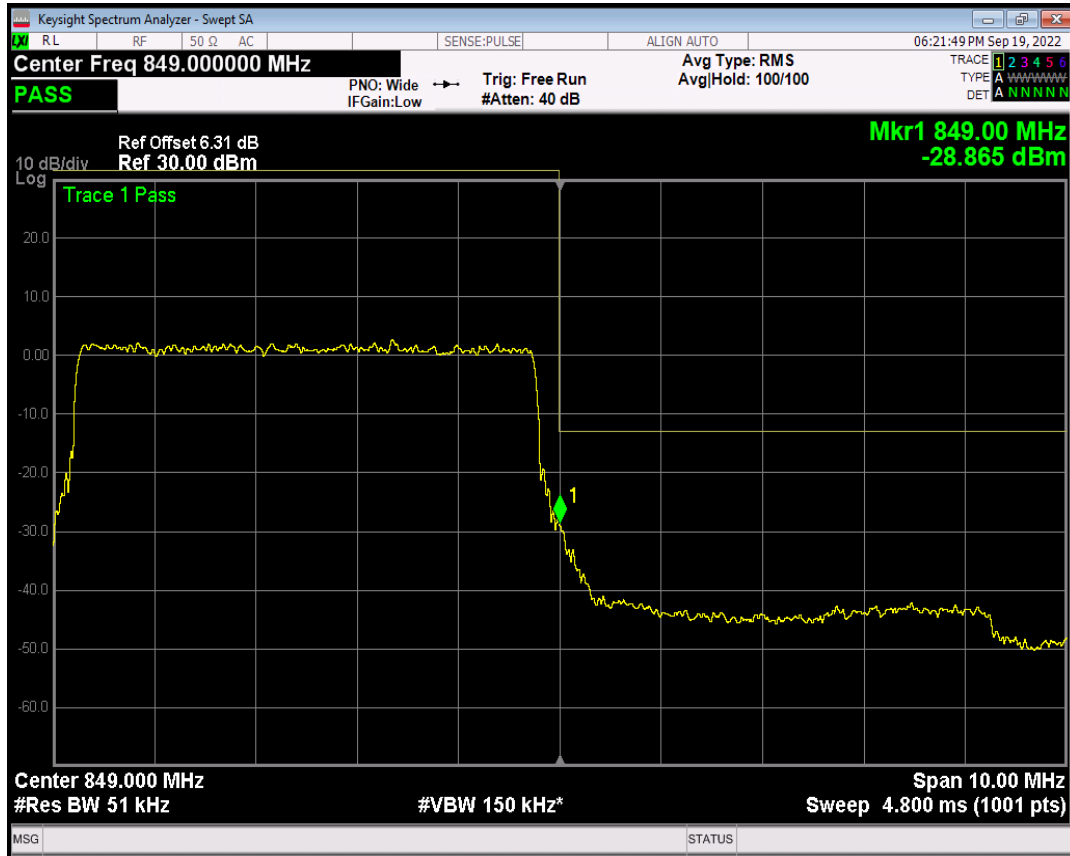
Band7 QAM16 BW=10MHz Channel=20800 RB Size=1 Position=#0
