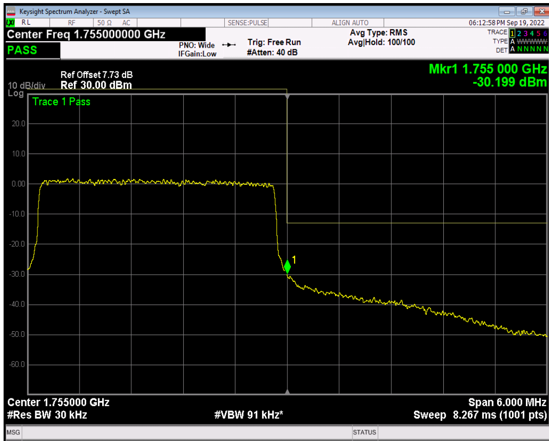
Band4 QAM16 BW=5MHz Channel=19975 RB Size=1 Position=#0
