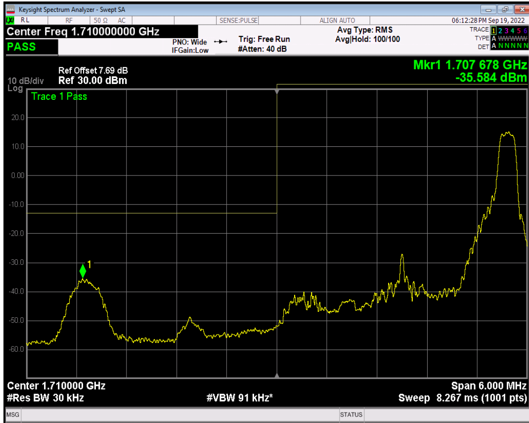
Band4 QPSK BW=3MHz Channel=19965 RB Size=15 Position=#0
