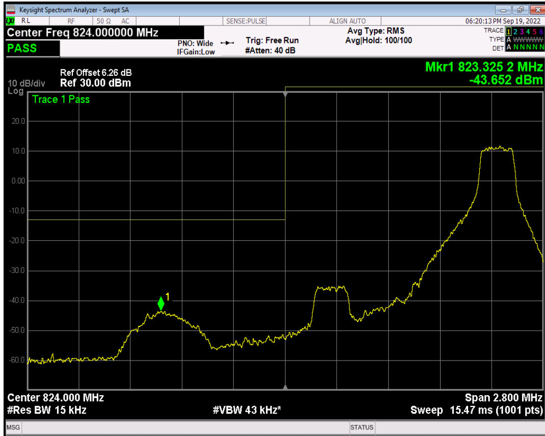
Band5 QPSK BW=1.4MHz Channel=20407 RB Size=6 Position=#0
