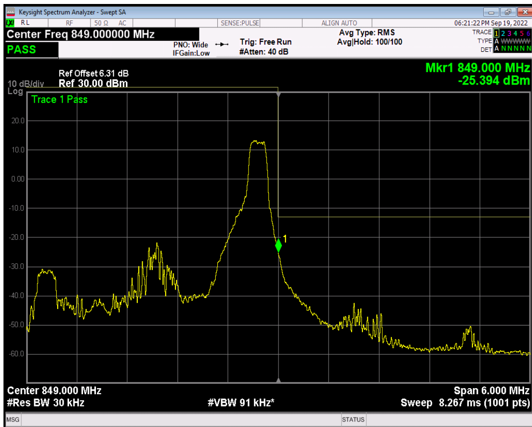
Band5 QAM16 BW=3MHz Channel=20635 RB Size=15 Position=#0
