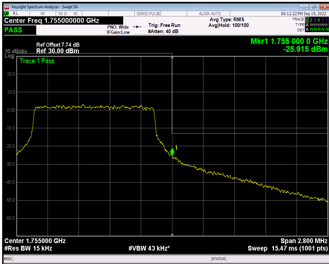
Band4 QAM16 BW=10MHz Channel=20000 RB Size=1 Position=#0
