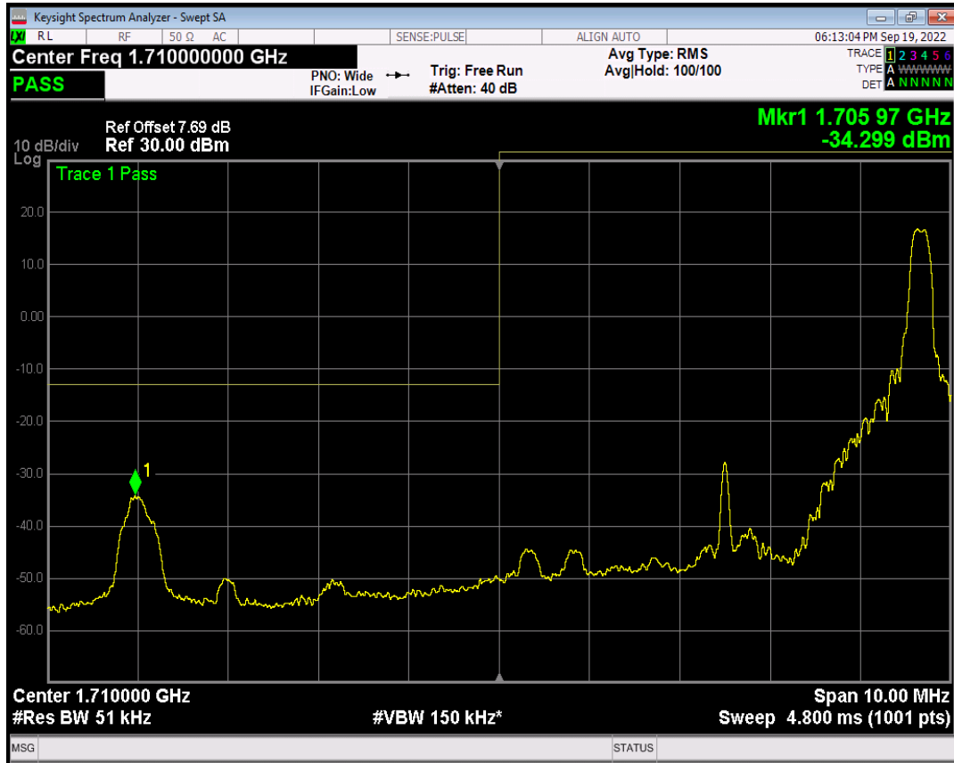
Band4 QPSK BW=5MHz Channel=19975 RB Size=25 Position=#0
