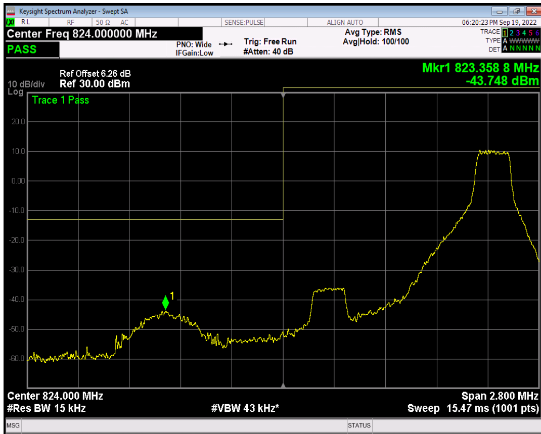
Band5 QAM16 BW=1.4MHz Channel=20407 RB Size=6 Position=#0
