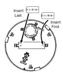
Install batteries in the sequence indicated. Use only 3 VDC CR123A batteries from the following approved sources:
