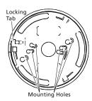
Secure backplate to the mounting surface using the screws provided. Note: Avoid mounting on uneven surfaces or electrical boxes. Warping of the backplate can result in a tamper.
