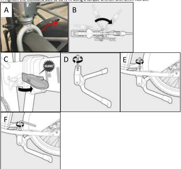
Marning: Failure to not secure the kickstand properly could cause it to fall off during riding.
