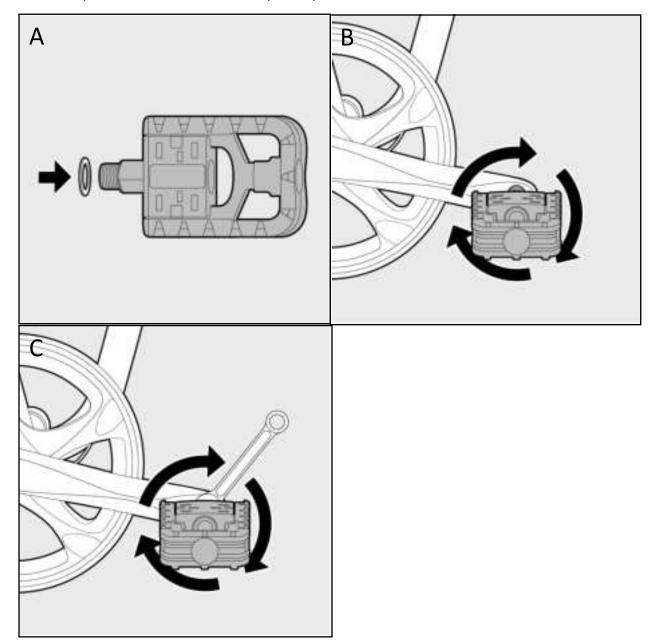
Note: We recommend applying pedal grease to the threads prior to installation. If replacing the left pedal, make sure to install the pedal while screwing counterclockwise.
