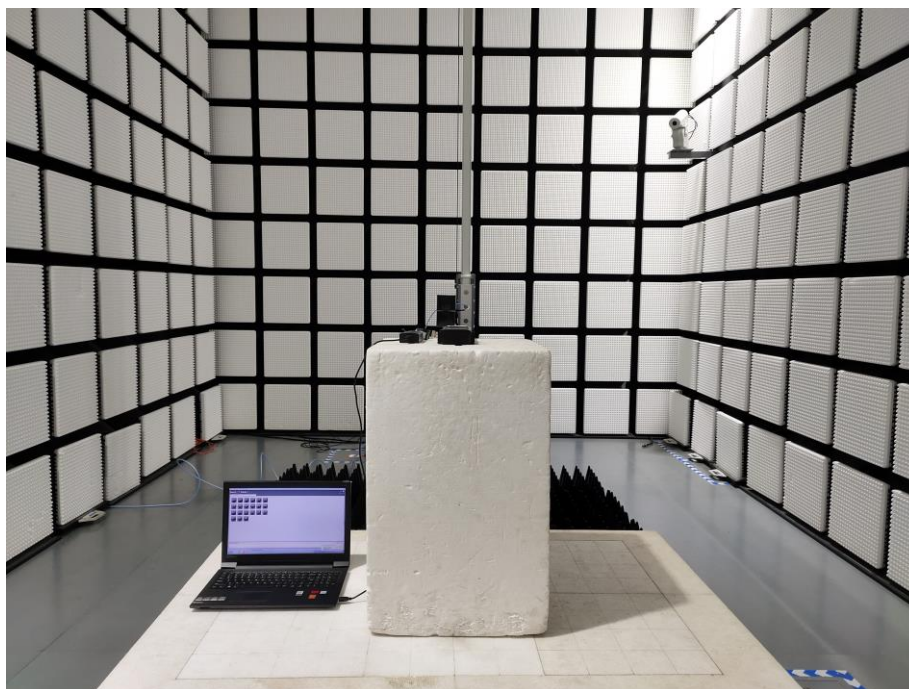
Fig. 3 Radiated emission setup photo(Above 1GHz)
