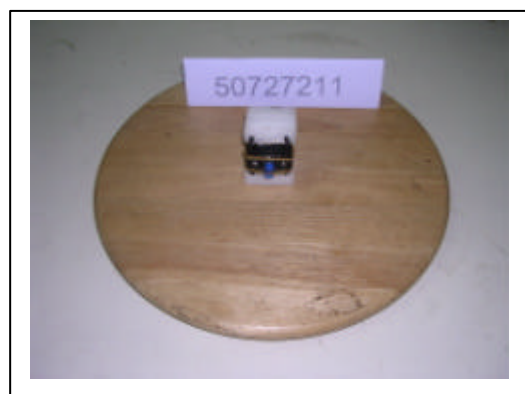
Radiated Open Site Test Set-up
