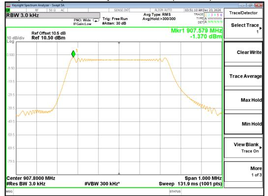
Screen Capture from Spectrum Analyzer: High Channel (DTS Mode)
