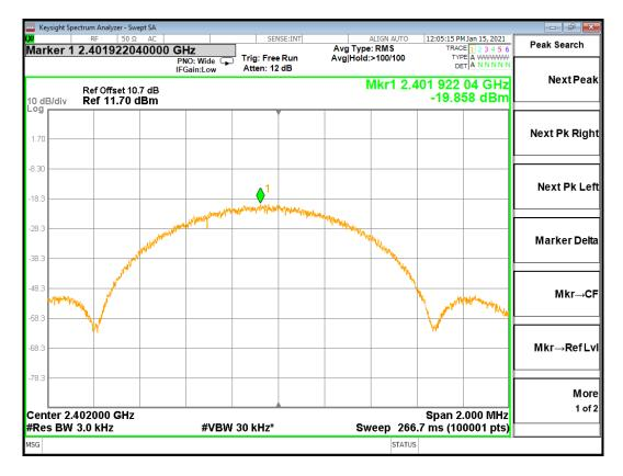
Screen Capture from Spectrum Analyzer: MID Channel (BLE)
