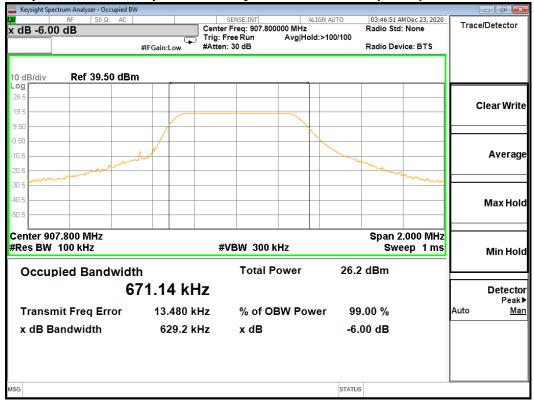
Screen captures from the spectrum analyzer High Channel (LoRA)
