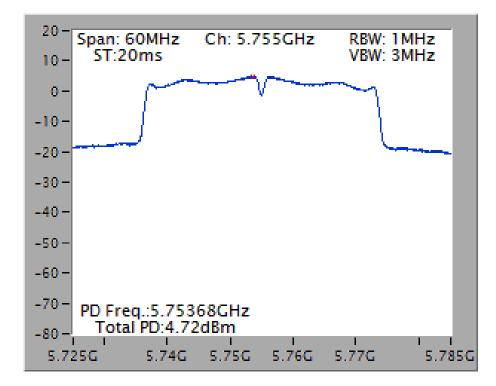
Power Density Plot on Configuration IEEE 802.11n MCS0 HT40 / Ant. 3 + Ant. 4 / 5755 MHz
