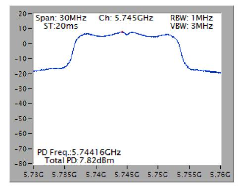
Power Density Plot on Configuration IEEE 802.11a / Ant. 3 + Ant. 4 / 5745 MHz
