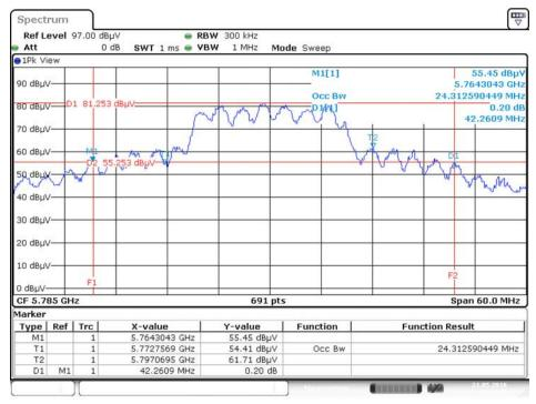
26dB Bandwidth and 99% Occupied Bandwidth Plot on Configuration IEEE 802.11n MCS0 HT20 / Ant. 3 + Ant. 4 / 5785 MHz
