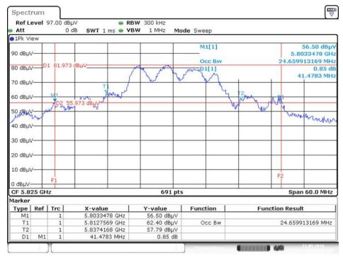
26dB Bandwidth and 99% Occupied Bandwidth Plot on Configuration IEEE 802.11a / Ant. 3 + Ant. 4 / 5825 MHz
