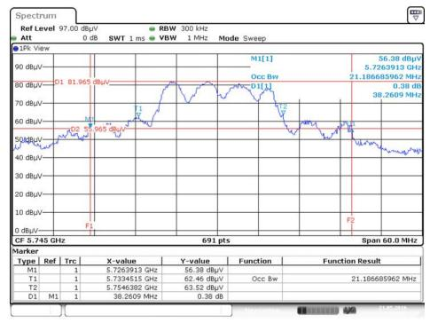
26dB Bandwidth and 99% Occupied Bandwidth Plot on Configuration IEEE 802.11a / Ant. 3 + Ant. 4 / 5745 MHz
