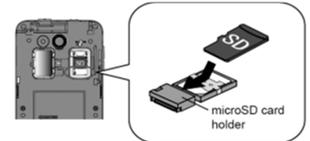
3. Close the SIM/microSD card holder cover and replace the back cover.
