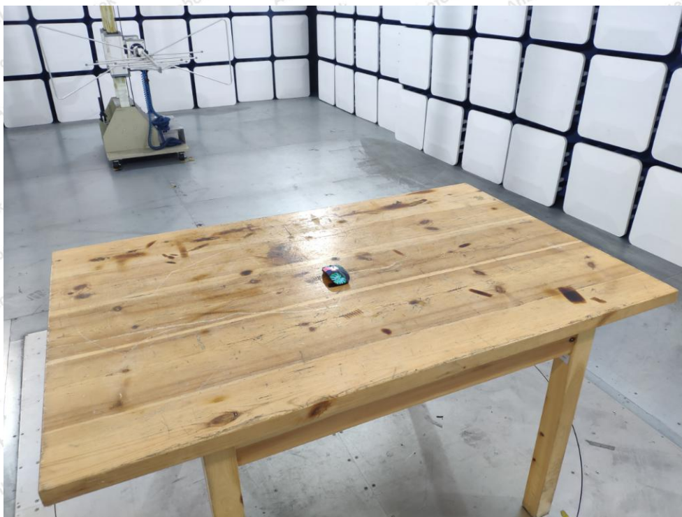
Photo of Radiation Emission Test
