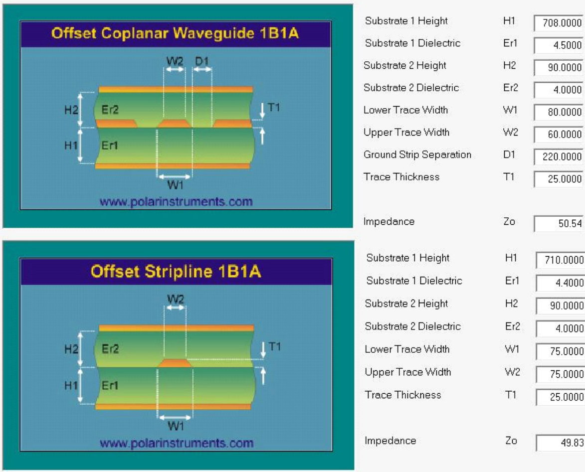
Figure 16: Embedded stripline arrangement example
