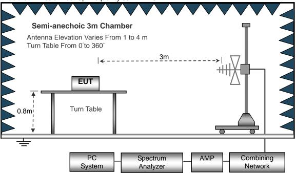
(C) Radiated Emission Test-Up Frequency Above 1GHz
